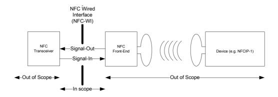
Figure 1 — Context diagram for the NFC wired interface
